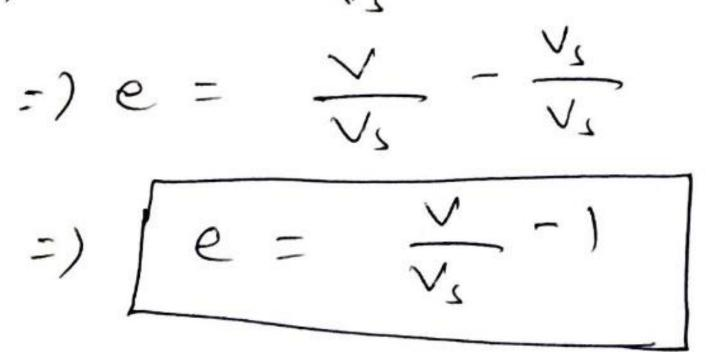
Porosity (n) The porosity n' of a soil sample is the ratio of volume of Noids to the total volume of given soil mass. Mathematically  $n = \frac{V_v}{V}$ =)  $n = \frac{V-V_s}{V} = \frac{V}{V} - \frac{V_s}{V}$
